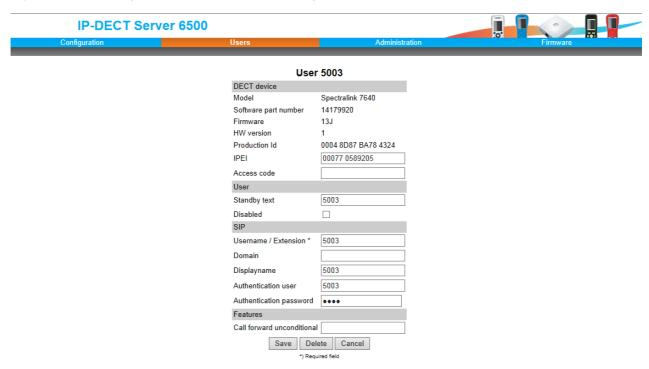
The data configured for each handset can be split into two categories. DECT data which is necessary for the correct handling of the DECT protocol stack. SIP data which is necessary for the handling of a SIP user agent.
